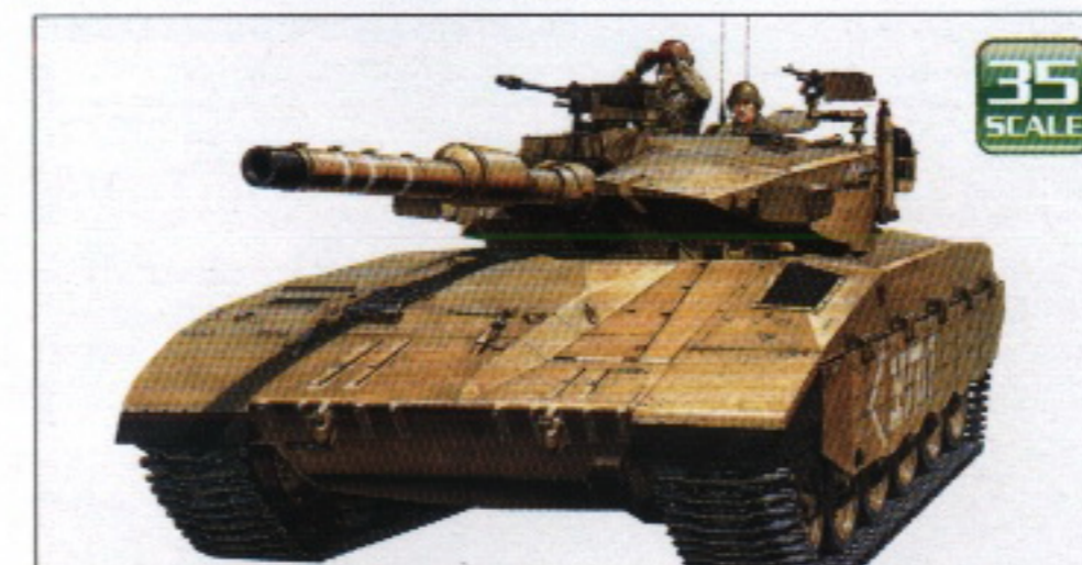
I.D.F. MERKAVA MK III 1391 The Merkava III differs from its predecessors in that it features a 120mm cannon and computerized fire control system that significantly increases accuracy.
